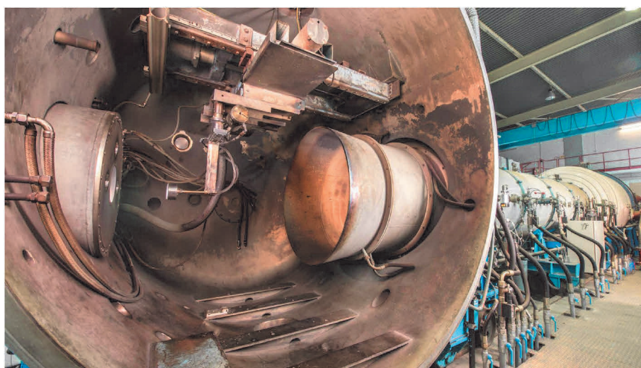
Fig. 5. L2K measuring chamber with nozzle flange, diffuser inlet, adjustment device, and test model. The sample in the figure is not linked to the SPADEXO test campaign. Credit: DLR (CC BY-NC-ND 3.0).
