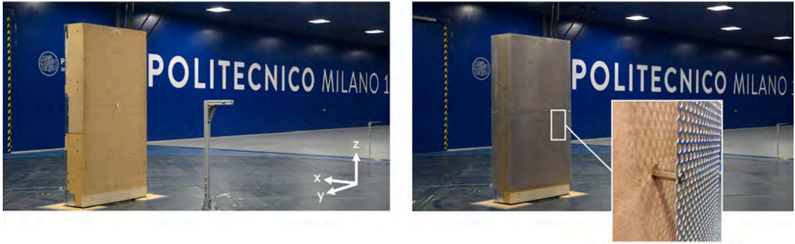
Fig. 1. Model in the wind tunnel test section. Left: naked configuration and reference system. Right: porous configuration, zoom on the porous envelope.
