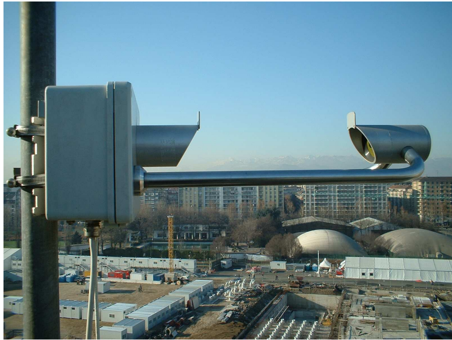
Fig. 1 – Thies-Clima disdrometer installed in Torino, C.so U.Sovietica 216
