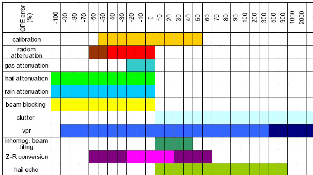
Figure 5.1: Range of relative errors (%) in radar QPE for a cell of 1 km x 1 km. Where the colours becomes darker are to be intended extreme values.
