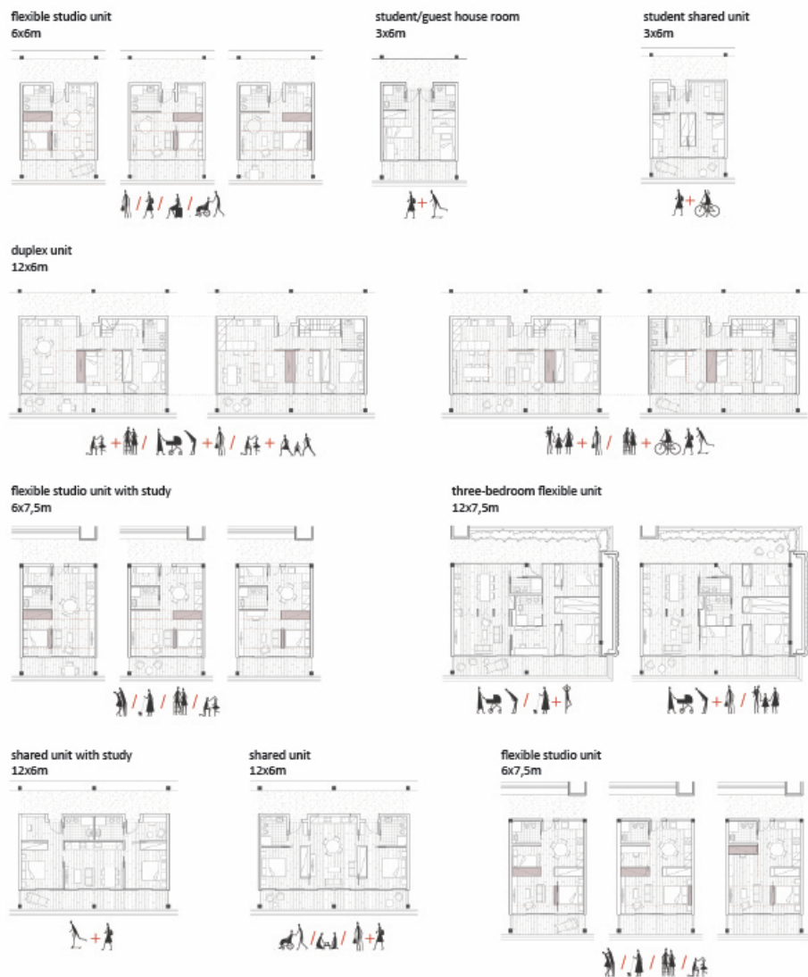
Fig. 20. Selection of typologies and possible modifications and users. (source: K. Tafaro and R. Farahbod, 2025)
