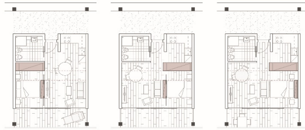
Fig. 19. 6x6 meters studio apartment unit with the flexibility of the inner partitions (source: K. Tafaro and R. Farahbod, 2025)
