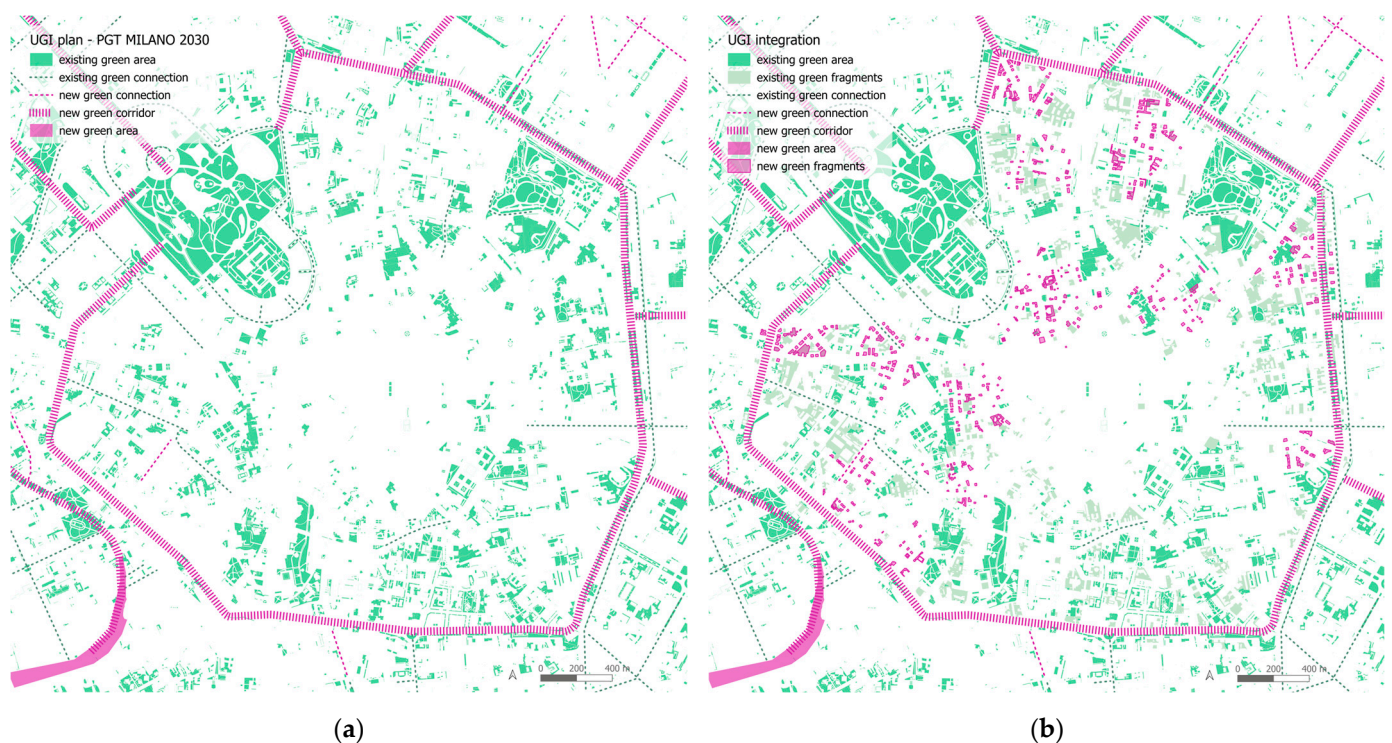
Figure 11. Complementarity of green network and green fragments approaches: (a) the current UGI program of PGT Milano 2030 surrounds the center but does not fit into it due to the spatial incompatibility of large-scale solutions in the compact urban matrix; (b) the proposed system of existing and potential green fragments complements the main network by ensuring good integration into the morphology of the historic center.
