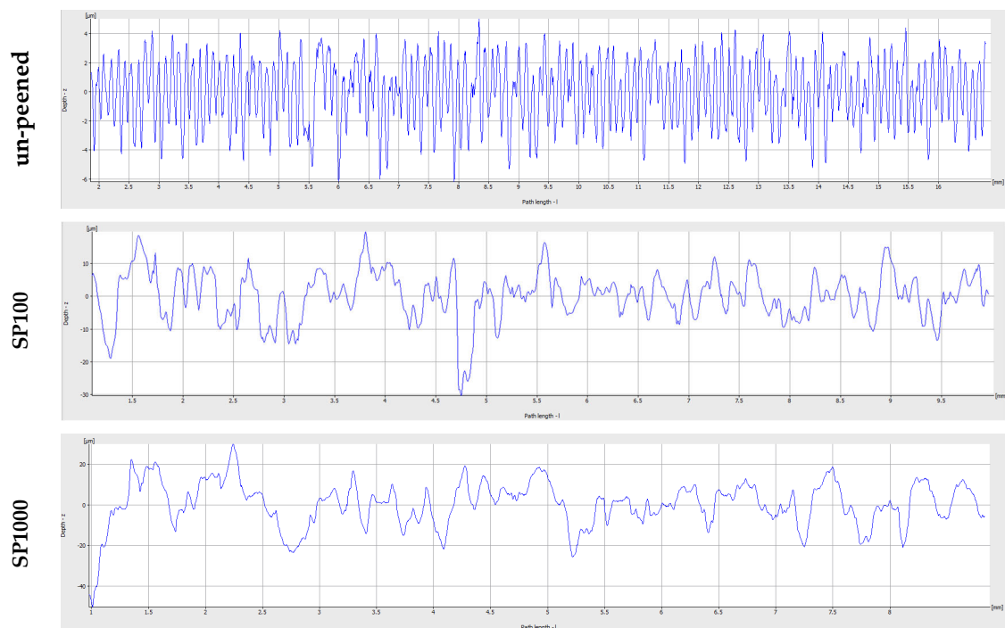
Figure 9. Surface roughness profiles of un-peened samples and samples after shot peening, varying by coverage levels ( \lambda_c = 2500 \mu\text{m} ).
