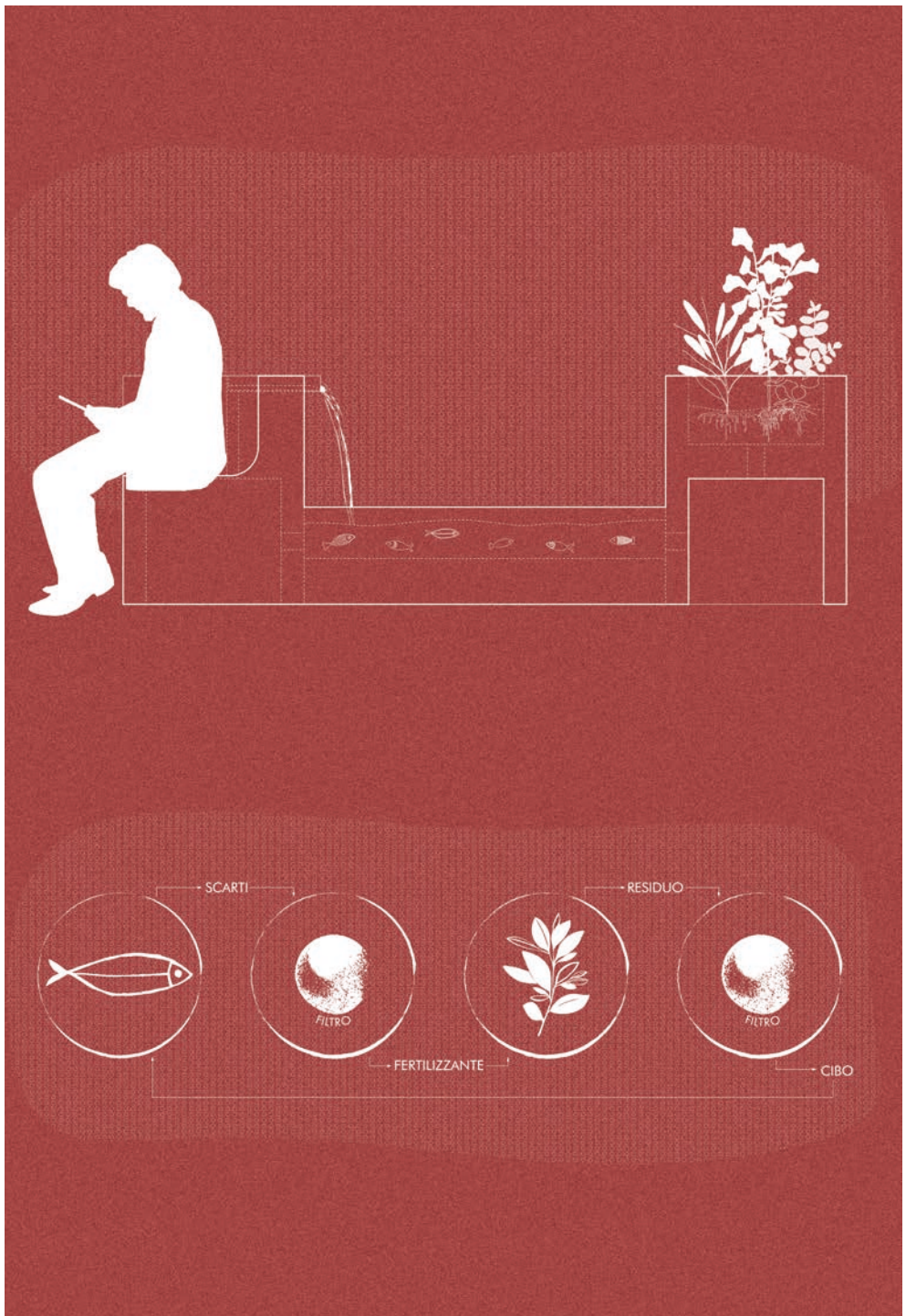
Vertical section of the device and diagram of the characteristic flows of aquaponic system. Metabolic waste from the fish is filtered into the plant tank, where it is transformed into nutrients by the bacteria present. The plants also contribute to increased comfort and/or local food production.
