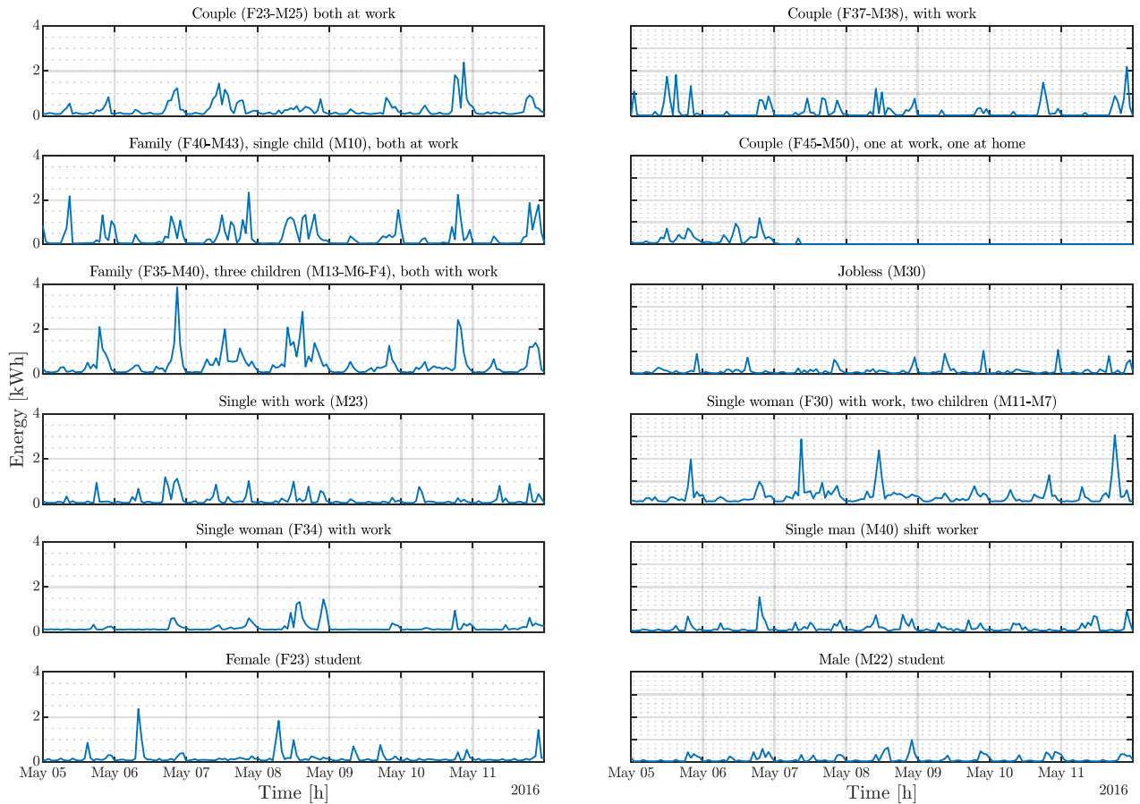
Figure 2. Example of electrical load profiles of the twelve apartments over one week
