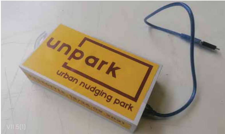
FIGURE VII.5 (1)(2)(3)- Some images of the mobile survey unit for particulate detection (PM 10 , PM 2,5 ), 2021 (Source: UNPark/ Matteo Clementi)
