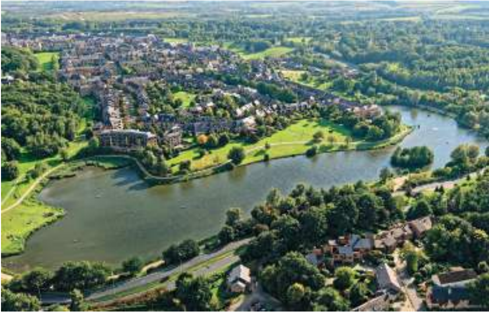
Figure 11. View (2019) of the rainwater reservoir treated as an artificial lake with variable water level, designed to attract high-density low-rise residential developments (source: Simon Schmitt, www.globalview.be ).
