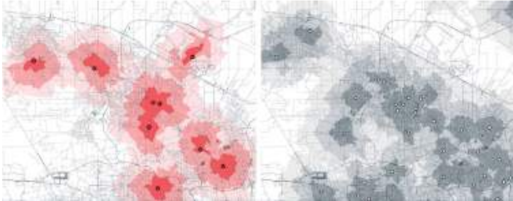
Figure 4. On the left 5, 10 and 15 minute isochrones according to train and metro stops. On the right according to high schools.
