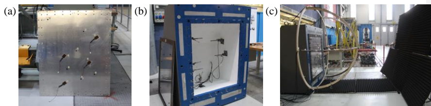
Fig. 1. Overall experimental set-up: (a) smart panel; (b) Noise-Box; (c) overall arrangement
