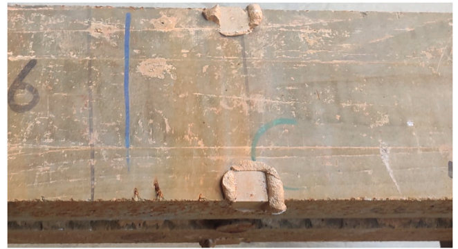
Fig. 12. Surface of a specimen exposed in geothermal water after twelve months.
