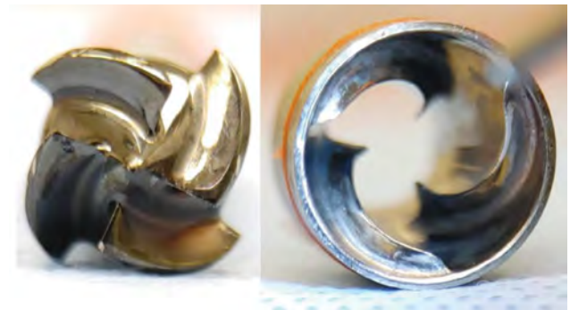
Explanted impeller and stator displaying freedom from thrombus deposition after 4 hours circulation in-vivo.
