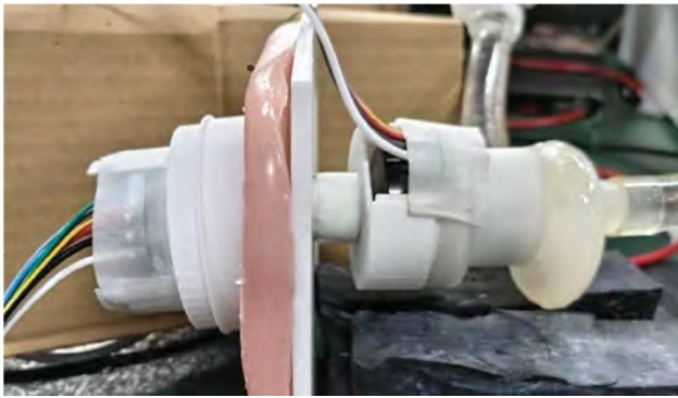
Picture of the new hybrid wireless left ventricular assist device.
