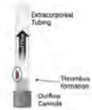
Figure 1. Generalized figure of a thrombus formation at the junction of the cannula and the tubing.
