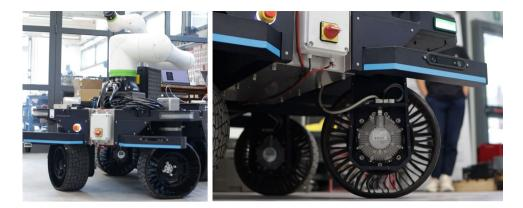
versatile and cooperating robotic platform for the creation of brick structures.
