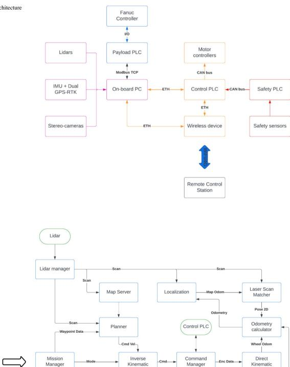
Fig. 7 Software architecture scheme
