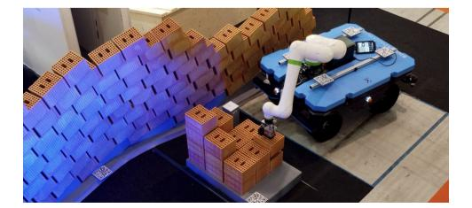
laborative, meaning they are built to work alongside construction workers, who play a crucial role in monitoring progress and ensuring everything runs smoothly. This integration is further enhanced using augmented reality to define safety zones and provide supervisory oversight, allowing for a seamless incorporation into existing practices (Fig. 3).
