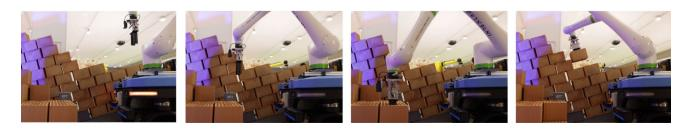
Fig. 12 Operation sequences of BRIX constructing a wall in Bari at SAIE fair 2023
