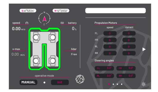
Fig. 11 Example of Rover HMI screen with telemetry
