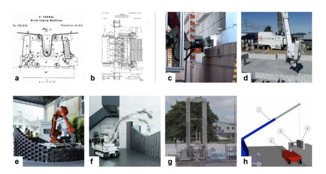
**Fig. 1** Principal innovations in bricklaying machines, from 1875 to 2023: **a** patent by C. Franke; **b** patent by J. Thomson; **c** SAM100; **d** Hadrian X; **e** DimRob; **f** in situ fabricator; **g** automated brick laying robot (ABLR); **h** crane+lightweight manipulator
