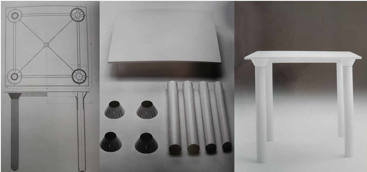
Fig. 3. Executive drawing and realization of squared Table 4300 and its realization. Kartell 1983–in production (images from Morozzi, pp. 108–110 [28]).
