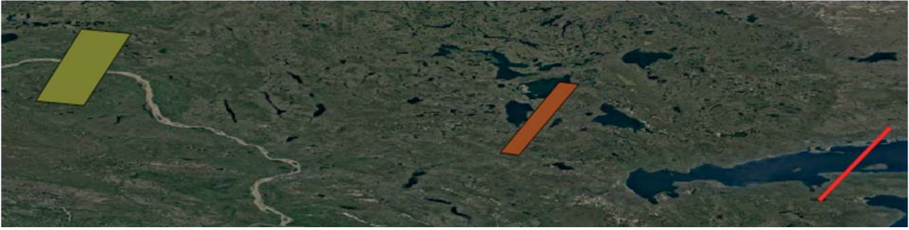
Figure 3 Geometry of ionosphere estimation: the acquired scene in yellow, ionosphere piercing area in orange, and the position of the satellite during acquisition is in red.
