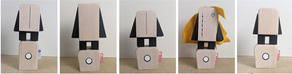
Fig. 4. Prototyping different design variations. Design elements such as the pedestal, capes, corps, arms, and legs were laser cut, glued together, and composed in different variations to be tested with the classification algorithm.
