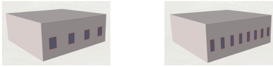
Fig. 2. Office south facade for WWR = 0.1 and a varying number of windows.
