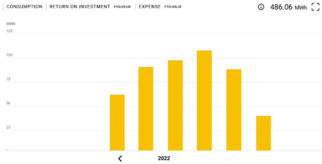
Figure 3: Monthly energy production by photovoltaic plant.
