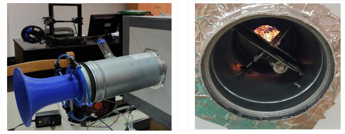
Figure 7: Flow rate valve located at the entrance of the experimental device.
