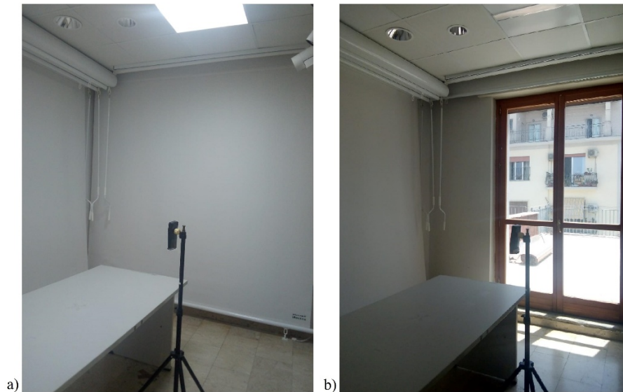
Fig. 4 – Photos of the room during electric light (a) and daylight (b) measurements for the configuration with the white wall
