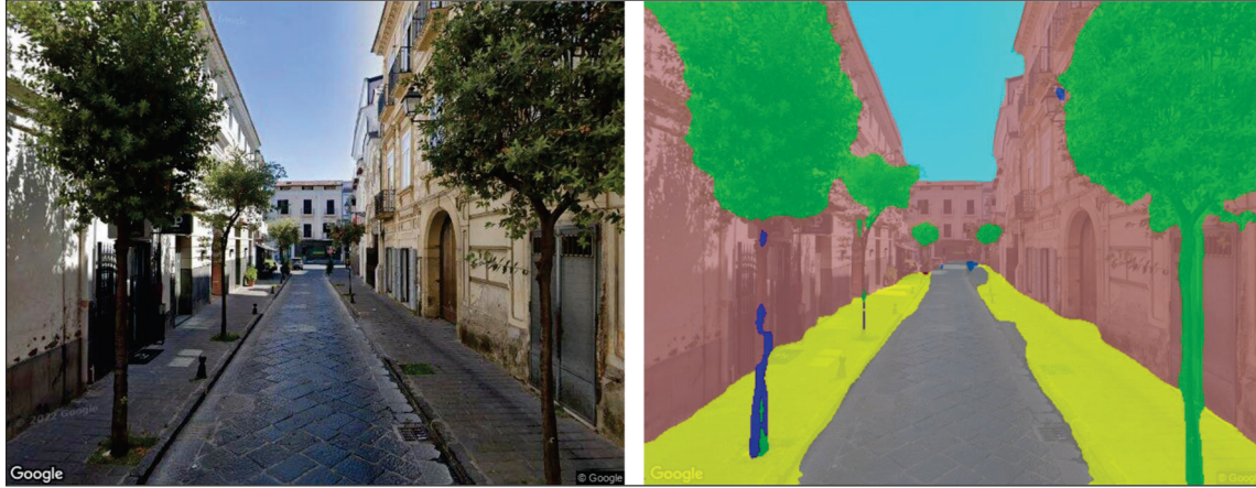
Figure 1. Comparison between the original Google Street View image and its semantic-segmentation output. The automated classification highlights all semantically detected classes by the DeepLabv3+ model.
