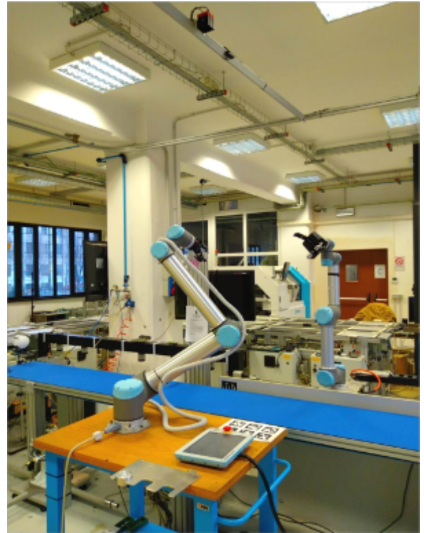
Fig. 1. Re-manufacturing pilot plant with the collaborative robot and the human-tracking system.
