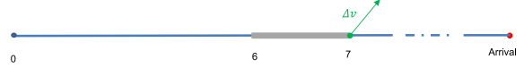
Fig. 3. M-ARGO transfer ConOps. The grey bars represents the OD phases, while the green arrows mark the TCMs points. Time in days after the departure time from L_2 .
