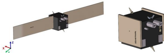
Figure 5. Zodiac Pioneer space vehicle concept, Payload and top decks (deployed and stowed configuration).
