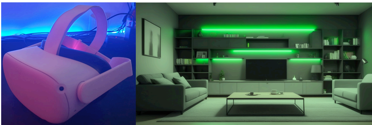
Fig. 2 - On the left, an adequately calibrated VR display could deliver coloured light to the test subjects. On the right is a mock-up of a typical living environment illuminated by dynamic coloured lights.
