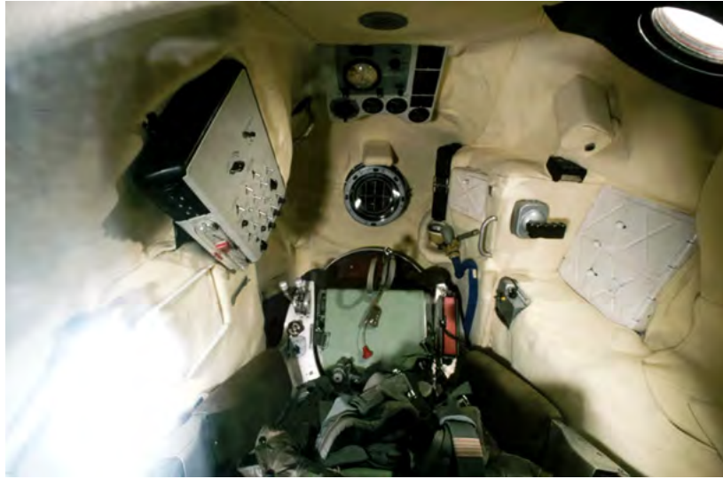
[1] Vostok 1. Interior of the habitat. The configuration is closed to cargo space rather than a habitable module in which the cosmonaut was fixed to the seat without the possibility to move. (Copyright Public Domain)
