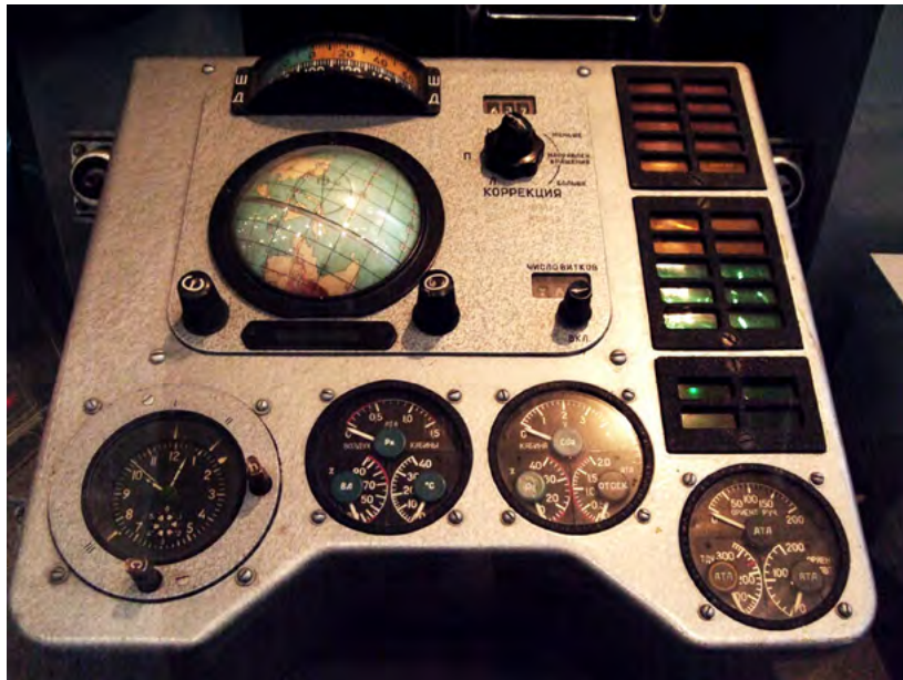
[2] Vostok 1. Control panel. It was placed in the center in front of the seat made of basic and rudimentary commands. (Courtesy Nasa History)
