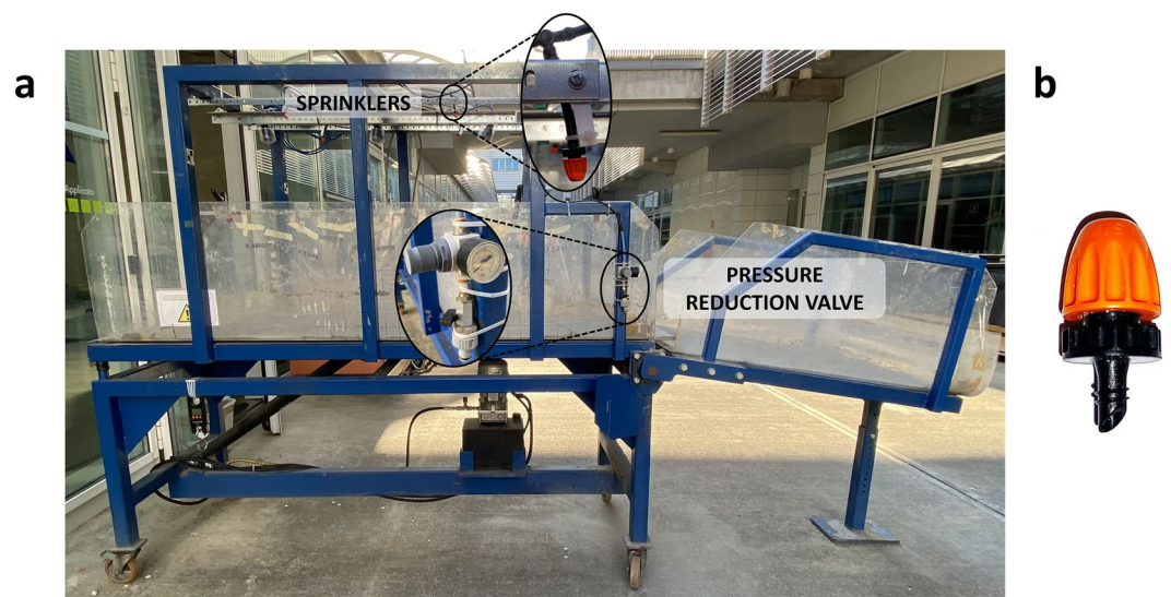
Fig. 4 (a) Rainfall simulation equipment installed on the landslide simulator with close-ups of a sprinkler and the pressure reduction valve. (b) Detail of a sprinkler.
