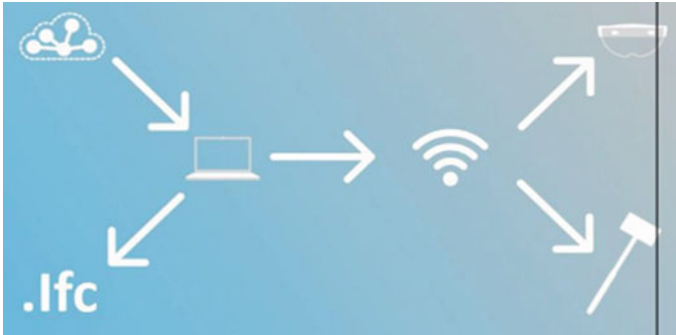
Fig. 4.2 The companion app prepares the point cloud to streaming and makes it available to the point cloud streaming service that is also running on the laptop. The laptop is then connected to a Wi-Fi that makes possible for other devices to stream and view
