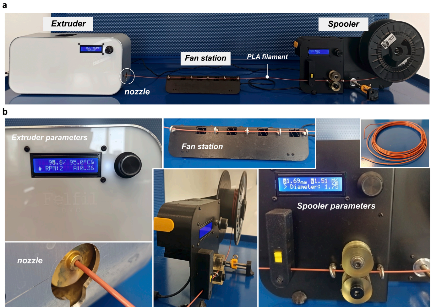
Fig. 2. An example of desktop-based filament extrusion technology by Felfil ( www.felfil.com ). a) The default configuration, from left to right, includes an extruder with its nozzle, a cooling station to solidify the extruded filament, and a spooler that checks the filament diameter and creates the spool. b) Some details of the extrusion technology presented in (a): main extruder parameters, the nozzle, the fan station, and the spooling system with its main parameters visible on a screen. The outcome, i.e., the filament, is also shown.
