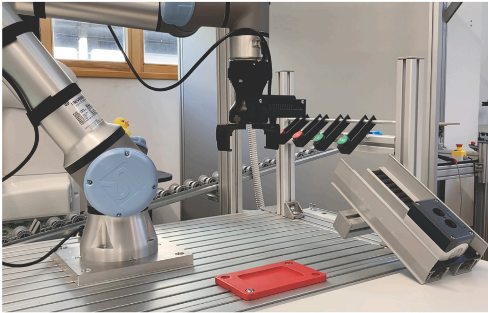
Fig. 5. Setup for the experimental validation. The case has to be picked from the bottom of the gravity feeder (right) and positioned on the red fixture. Four different buttons are arranged into four gravity feeders (right). (For interpretation of the references to colour in this figure legend, the reader is referred to the web version of this article.)
