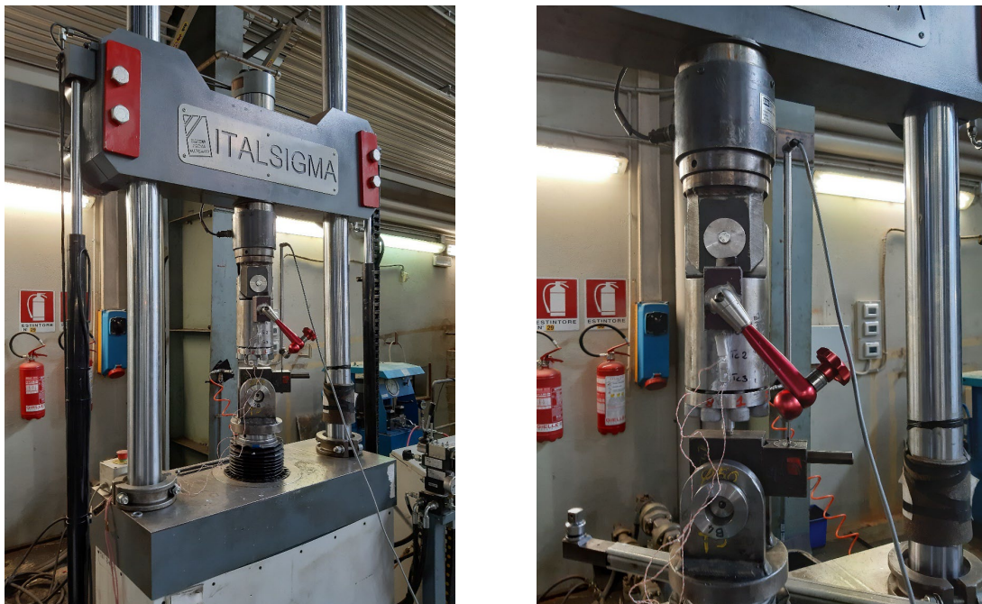
Figure 4. Test specimen installed on the testing frame (left) and close-up view (right), with details of connections at the spherical hinges and the external displacement transducer.
