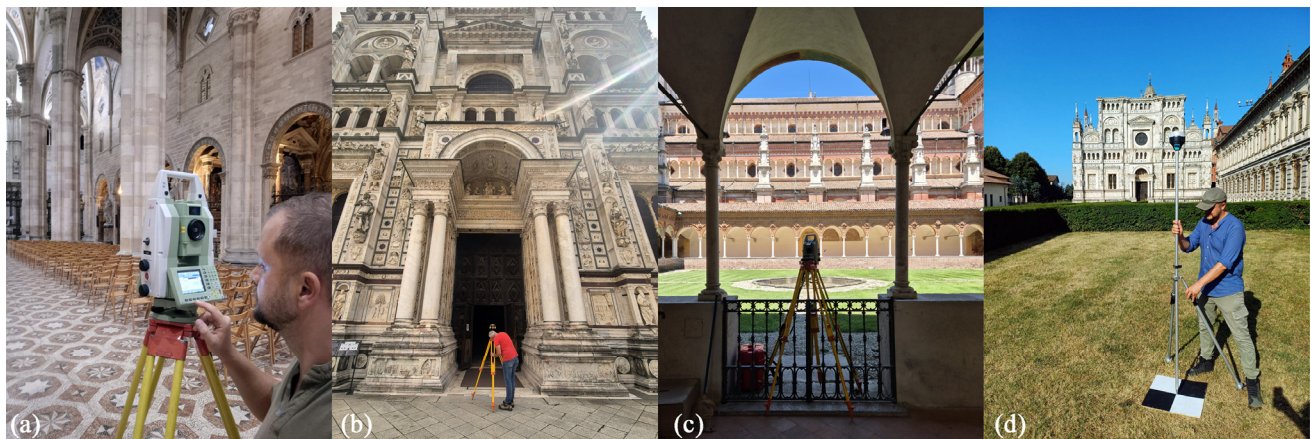
Figure 7. Topographic survey operations at the Certosa di Pavia: (a) nave; (b) main entrance of the church; (c) Small Cloister—survey carried out using a Leica TPS1203 total station; (d) church forecourt—GNSS RTK survey conducted using an Emlid Reach RS3 receiver.
