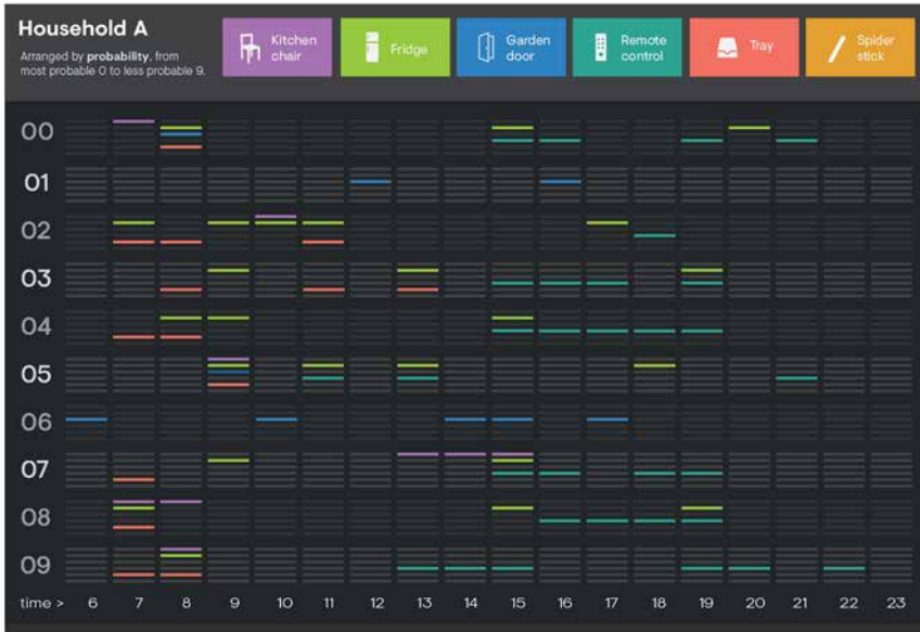
FIGURE 6.11 Resourceful Ageing: Visualization of machine learning interpretation of the co-usage of objects, from high to low probability of occurrence. Data visualization by Philips Design.
