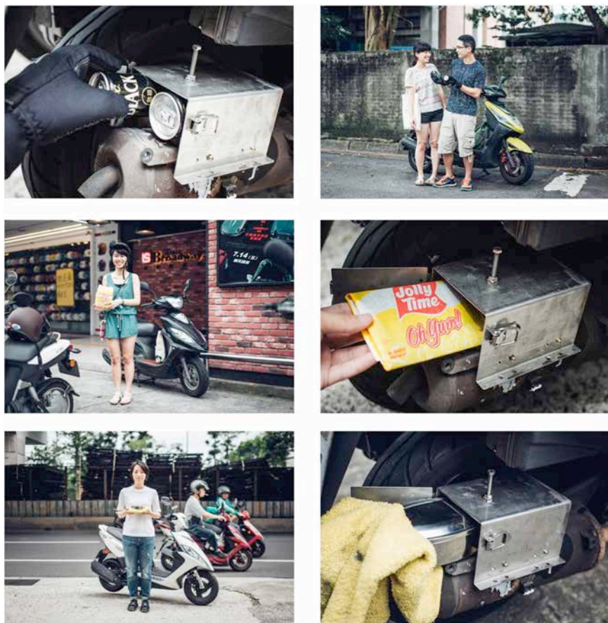
FIGURE 6.3 Pipe heater is the speculative concept for an open-ended device that reuses the heat produced during a ride for personally and socially meaningful activities (e.g., warming up food, sharing a hot drink). Photos by Wen-Wei Chang.
