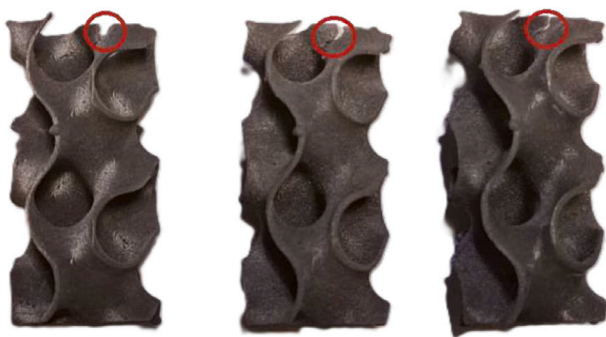
Fig. 14. F2_GY rupture point.
