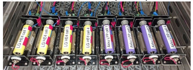
(b) Li-Ion battery cells: four NMC (yellow) and four LFP (blue).
