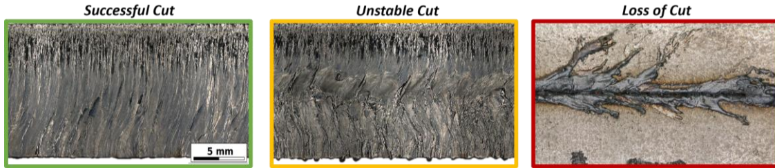
Figure 2: Qualitative cutting results for 20 mm thick AISI304: Loss of Cut (in red); Unstable Cut (in yellow) and Successful Cut (in green).
