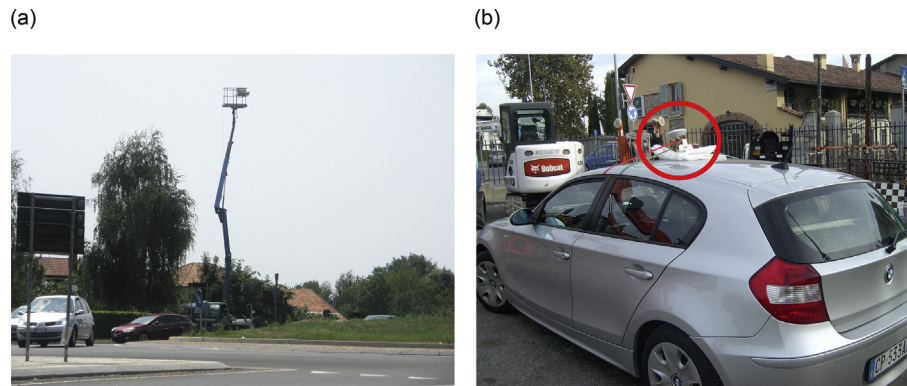
Fig. 2 – Data collection and evaluation instrumentation. (a) Vision system placed upon a raised working platform. (b) The probe vehicle with the rover system.
