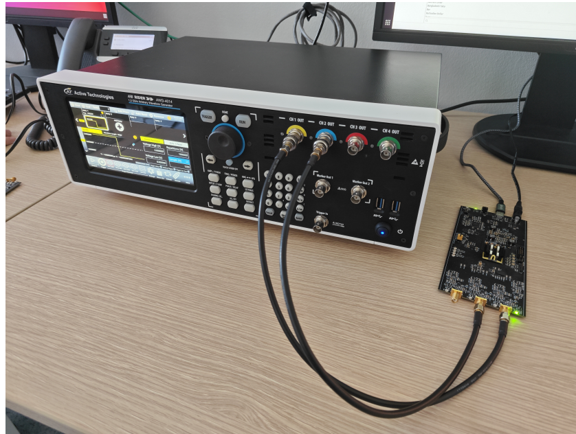
Figure 16. Experimental setup with the ACTIVEAWG401X on the left and FELIX module on the right.
