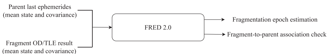
Fig. 2. General flow chart of the epoch estimation algorithm of FRED 2.0.
