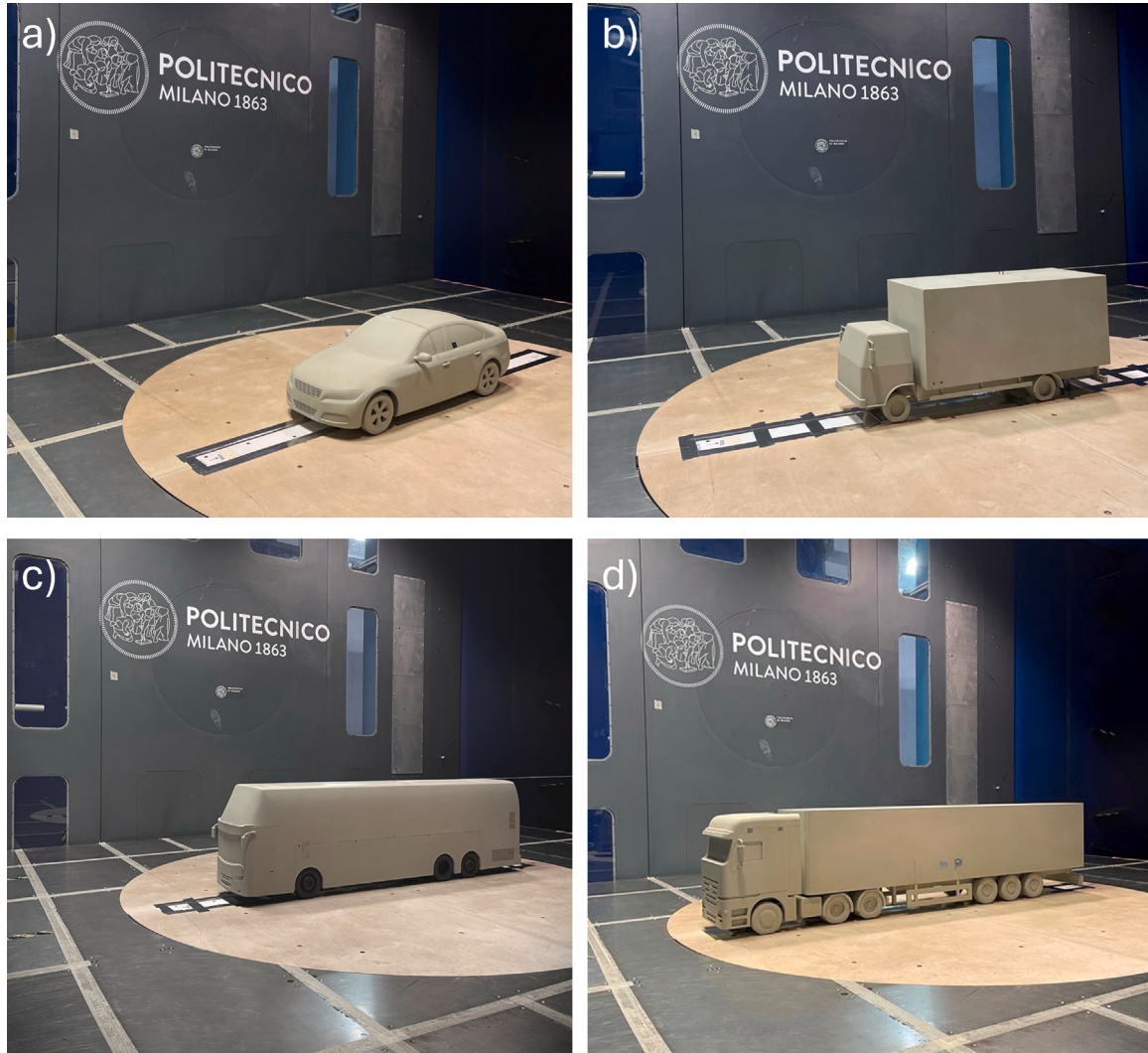
Fig. 2. Vehicle models mounted in the Politecnico di Milano wind tunnel during the experimental campaign: (a) saloon car (DrivAer), (b) small lorry, (c) double-decker coach, (d) articulated lorry. All models are tested on the turntable under flat-ground conditions; the mounting arrangement is designed to minimise aerodynamic interference in the underbody region.
