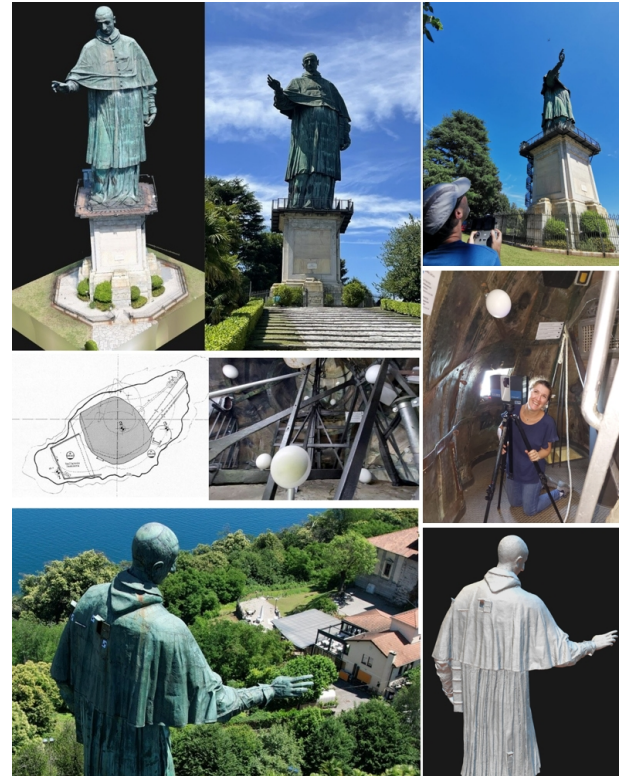
Figure 2: Documentation through surveying and modelling: overview of the 2022 campaign.
