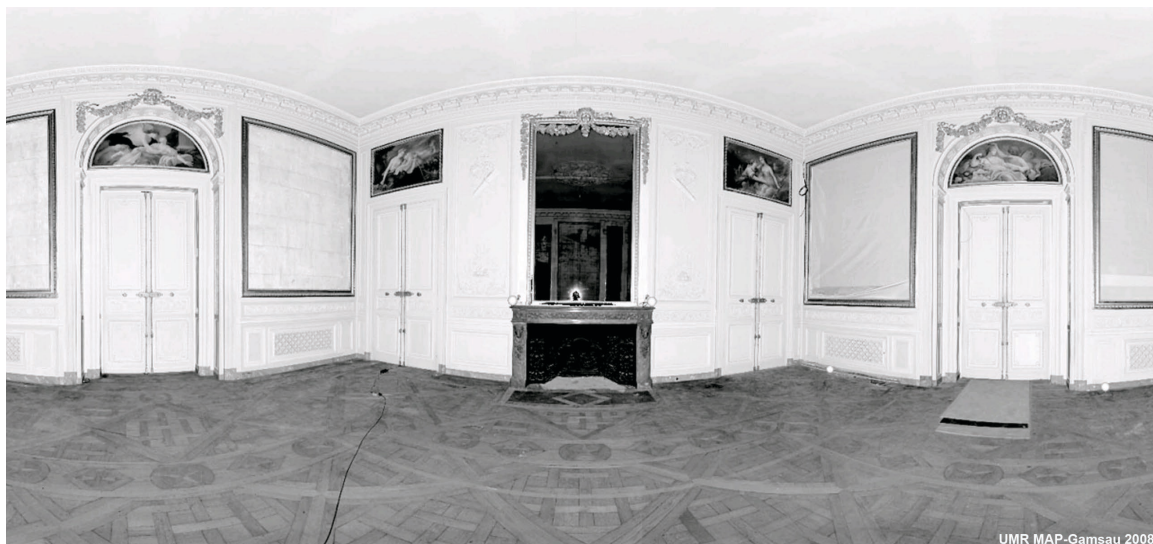
Fig. 1 Point cloud obtained by laser scanning of room.
