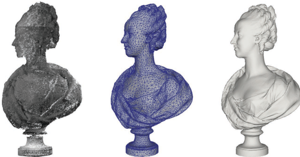
Fig. 3 Steps of laser-based modelling: point cloud, geometry, ambient occlusion render.
