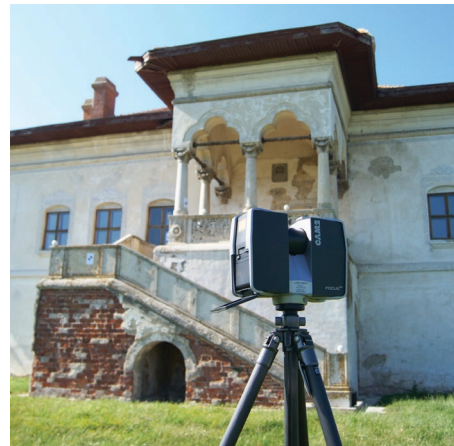
Fig. 18 3D outdoor laser scanner survey operation.
