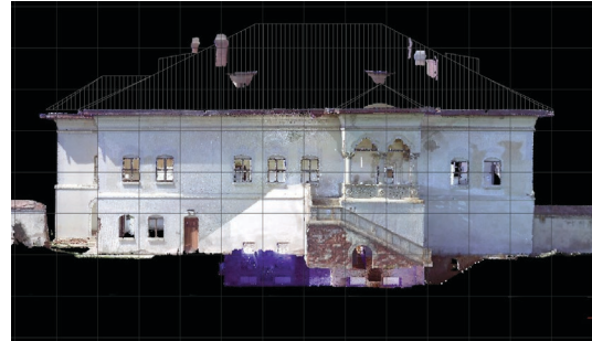
Fig. 29 South elevation (grid spacing 3 m).
