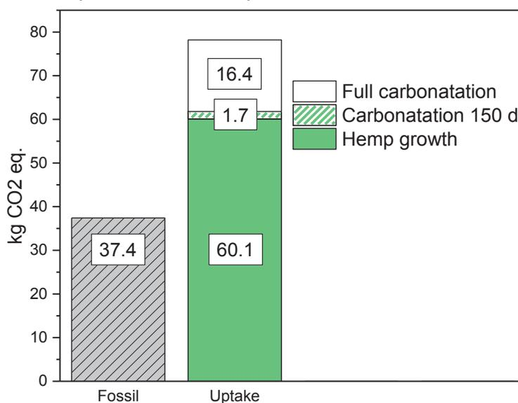
Figure 6:  $\text{CO}_2$  fossil emissions vs uptake (FU: 1 m<sup>2</sup> hempcrete wall)
