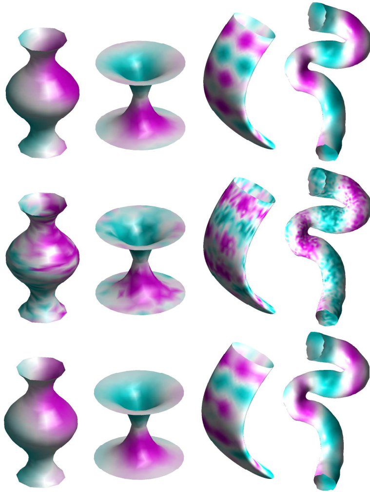
Fig. 4. Simulation study. Top: colormap of a test function generated by (21) on four tubular domains; the fourth one is a real geometry of an internal carotid artery from the AneuRisk dataset. Middle: data with noise. Bottom: estimates provided by the spatial regression model over non-planar domains. The colormap range is optimized for each geometry, magenta to green (min,max); Geometry 1: (-4.06, 6.06) ; Geometry 2: (-0.79, 2.79) ; Geometry 3: (-5.14, 7.17) ; Geometry 4: (-2.09, 4.10) .
