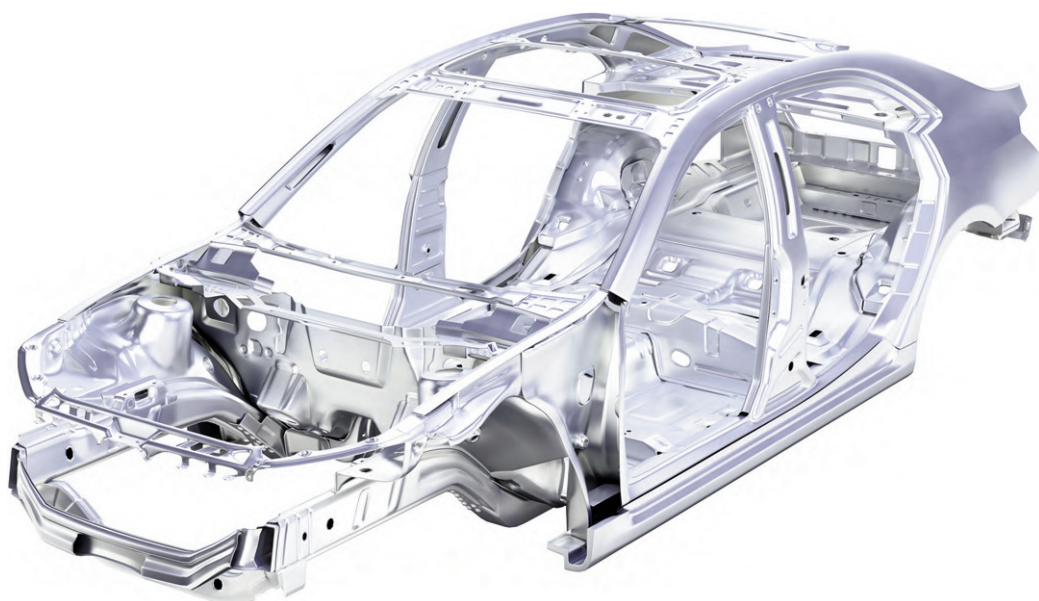
Fig. 1 | BIW design and monocoque structure (credit: Kutz, 2011).
