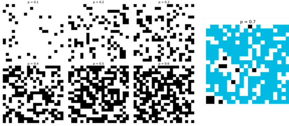
Fig. 4. As the absence probability p increases, the retained connectivity decreases. Below the critical absence threshold, a system-spanning load path can still persist, whereas above it, the network tends to fragment and the load-transfer capability is progressively lost.
