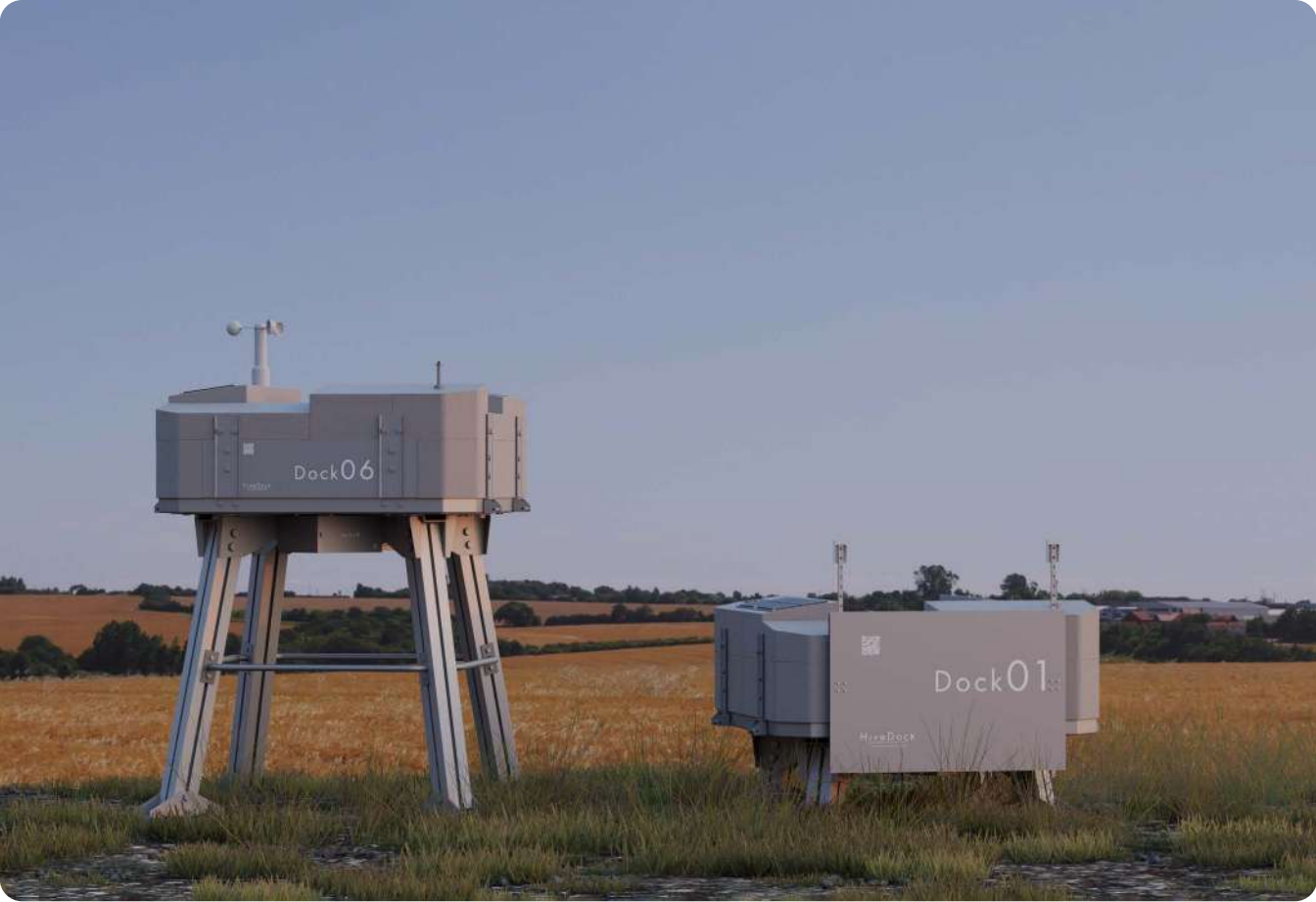
Image 1 Two HiveDock stations: the one on the left is designed for aerial platforms, while the one on the right has been adapted for ground platforms.
