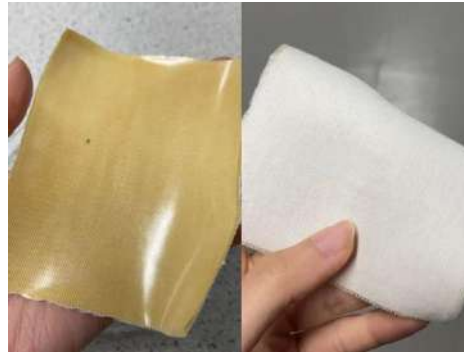
Figure.5 Direct film casting cotton (front and back)
