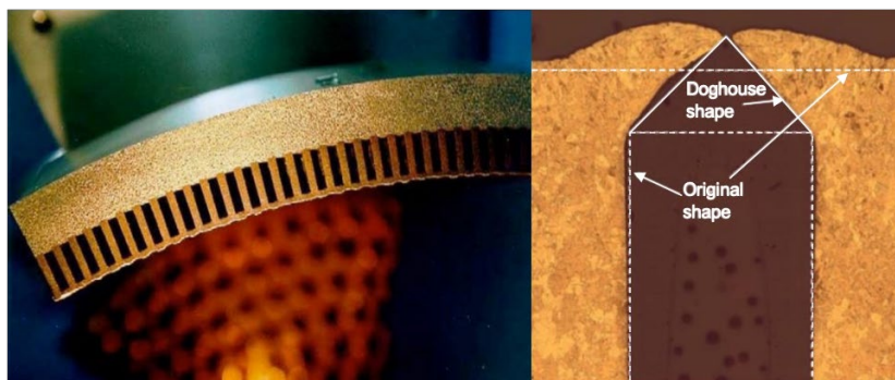
Cut through a Cu-based combustion chamber wall with representative micrograph of the cross section after failure.
