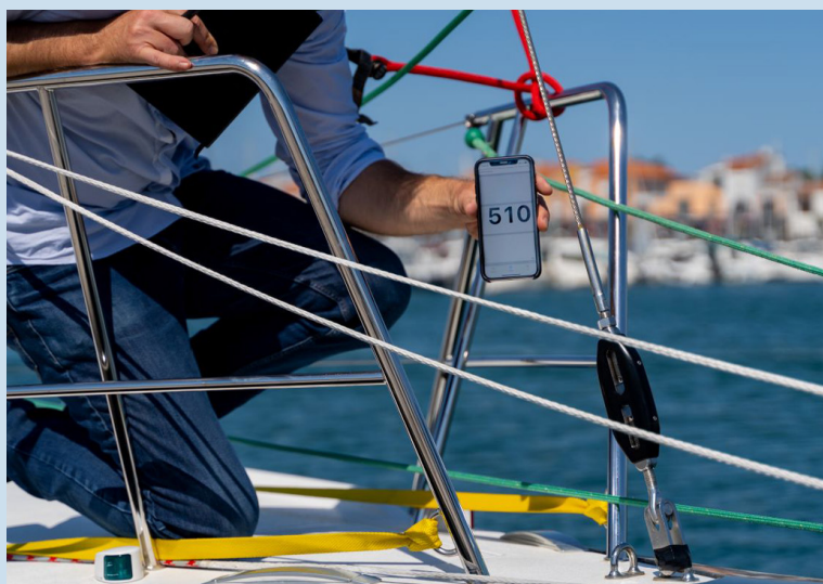
Figure 5. Cyclop Marine load sensing technology for standing rigging. Credits: Cyclop Marine Ltd.
